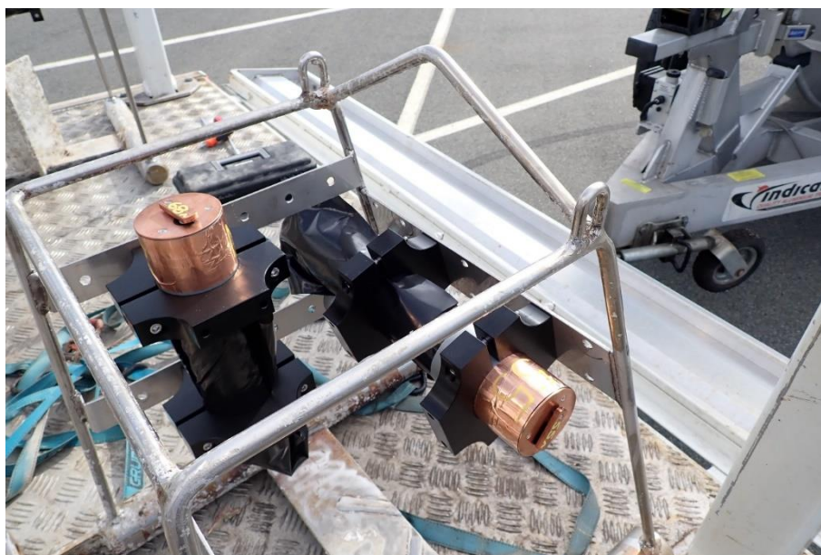
Figure 2. Turbidity and light loggers attached to instrument frame ready for deployment on the seafloor.
