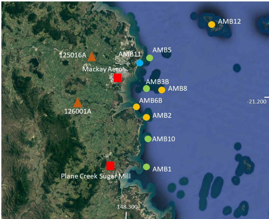
Figure 1.1 Location of water quality monitoring sites with loggers (green circle), without loggers (blue circles), and sites decommissioned (yellow circles) utilised in the 2020-2021 reporting period (exception of AMB6B which is PAR only and reported with seagrass reports). Also shown are meteorological stations (red square), and stream gauging stations (orange triangle) referred to in this report.
