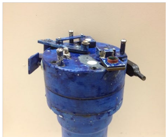
Figure 2.2 Example coastal multiparameter water quality instrument: a) site navigation beacon for safety and instrument retrieval; b) instrument showing sensors and wiping mechanisms
