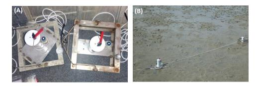
**Figure 11.** (A) Logging station consisting of a stainless steel frame with PAR loggers and temperature loggers attached, and wiper units; (B) example of deployment of logging stations (Abbot Point stations are subtidal only).
