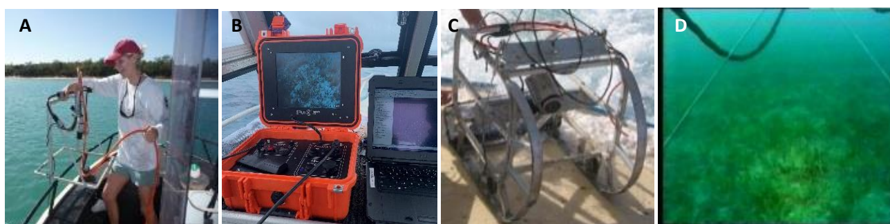
Figure 6. (A-B) Shallow subtidal assessments of seagrass meadows using digital camera mounted on a 0.25m 2 drop frame, and (C-D) offshore underwater sled tows with digital camera.
