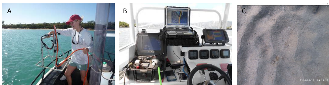
Figure 2. Benthic habitat assessments using live feed digital cameras and spatial referencing equipment.
