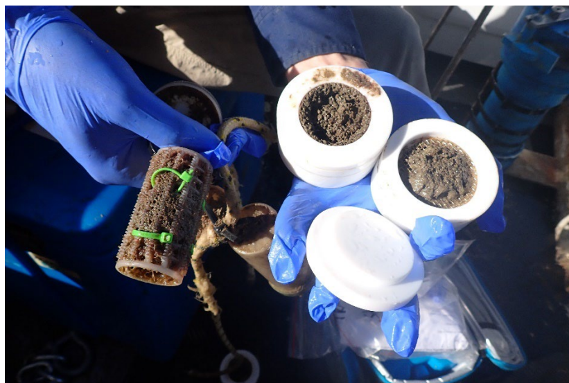
Figure 2-2. Pesticide monitoring passive samplers such as these were retrieved from Aquila Island (MKY_CAM1) in December, February, March, and June of the reporting period (Table 2-5). Note: biological growth on the samplers.
