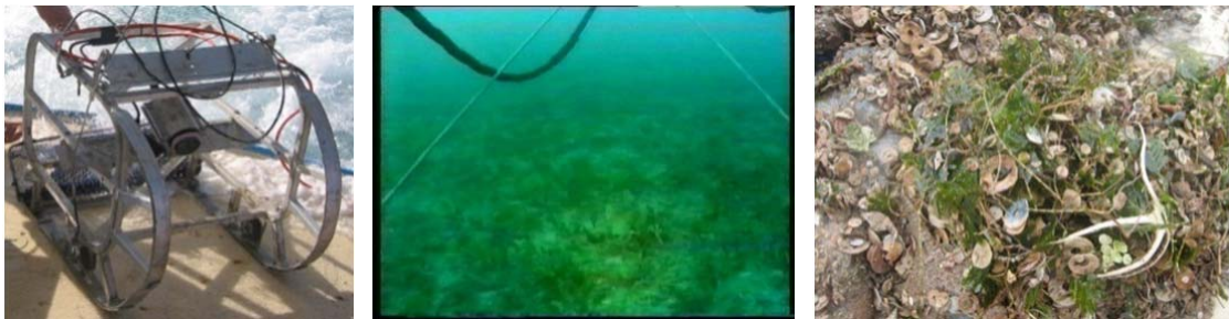
Figure 2 Deep water sled tows using CCTV system and sled net.
