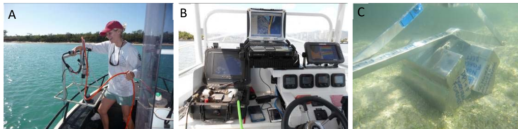
Figure 2. Benthic habitat assessments using (a & b) live digital camera and (c) Van Veen sediment grab.
