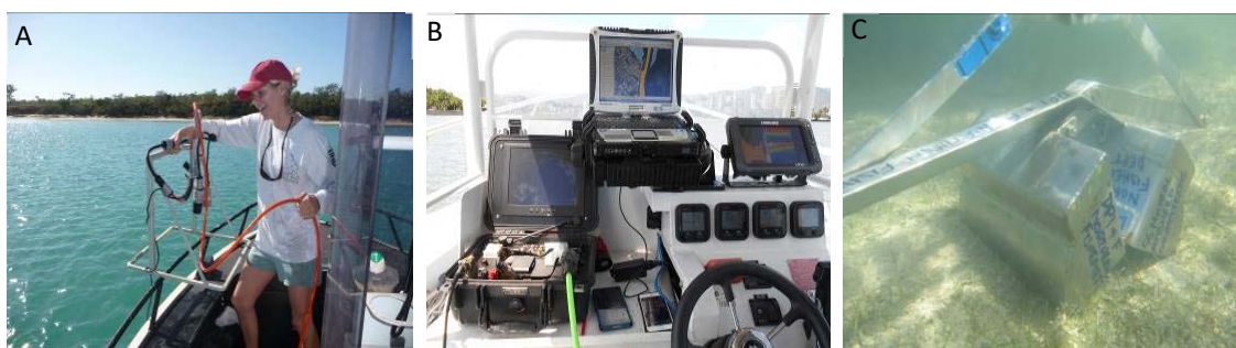
Figure 2. Methods used for marine macrophyte habitat assessments using (A & B) live digital camera and (C) Van Veen sediment grab.
