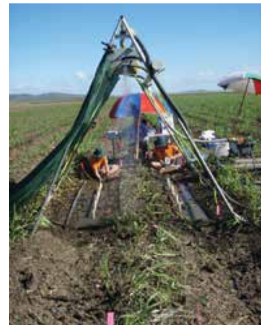
Spot spray rainfall simulation trials were conducted to examine the potential for improved spray technology to reduce surface runoff losses of herbicides from cane paddocks
