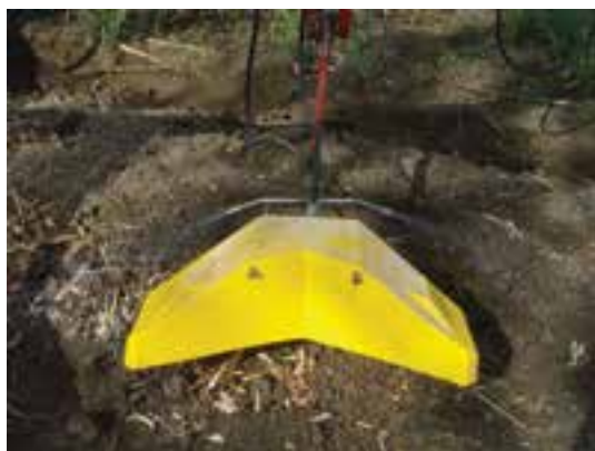
Close up of a shielded spray applicator which reduces runoff of herbicides by 90%
